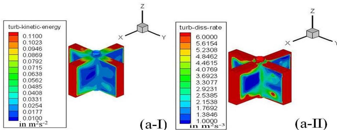
Figure 4: Contour of (a-I) turbulent kinetic energy and (a-II) turbulence dissipation energy at TMP = 588.kPa and  $\Omega = 41.9 \text{ rad s}^{-1}$ .
