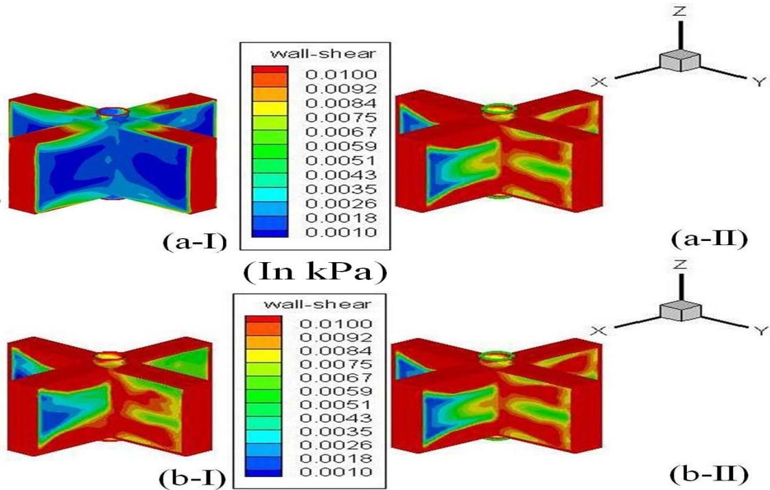
Figure 3: Contour of wall shear stress on basket surface (a) at different speed (TMP = 588.4 kPa): (I)  $10.47 \text{ rad s}^{-1}$  (II)  $41.9 \text{ rad s}^{-1}$  and (b) at different TMP ( $\Omega = 41.9 \text{ rad s}^{-1}$ ): (I) 98 kPa (II) 588.4 kPa.
