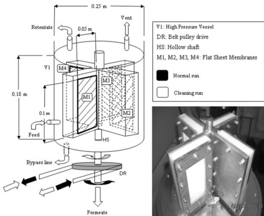
Figure 1: Schematic diagram of the Spinning Basket Module (insert showing a photograph of the spinning basket)
