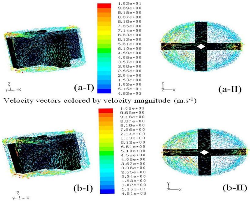
Figure 2: Distribution of velocity vector in default interior of SBM module for (a-I) and (a-II)  $\Omega = 10.47 \text{ rad s}^{-1}$  and TMP = 588.4 kPa, (b-I) and (b-II)  $\Omega = 41.9 \text{ rad s}^{-1}$  and TMP = 588.4 kPa.
