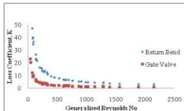
Figure 4: Plot of Loss coefficient (K) vs. Generalized Reynolds No. (N<sub>RE</sub>\*)
