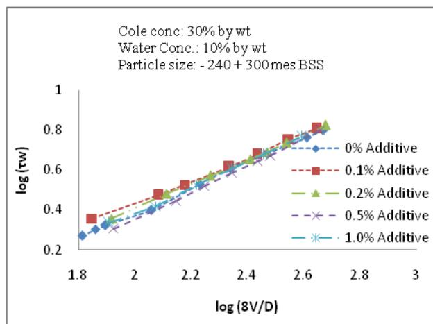
Figure 3: - Variation of log (τ<sub>w</sub>) with log (8V/D) for coal oil water slurry with additives
