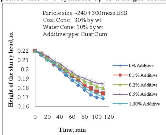
Figure 1: Variation of height of slurry head with time for different gaur gum concentration of coal – oil water slurry
