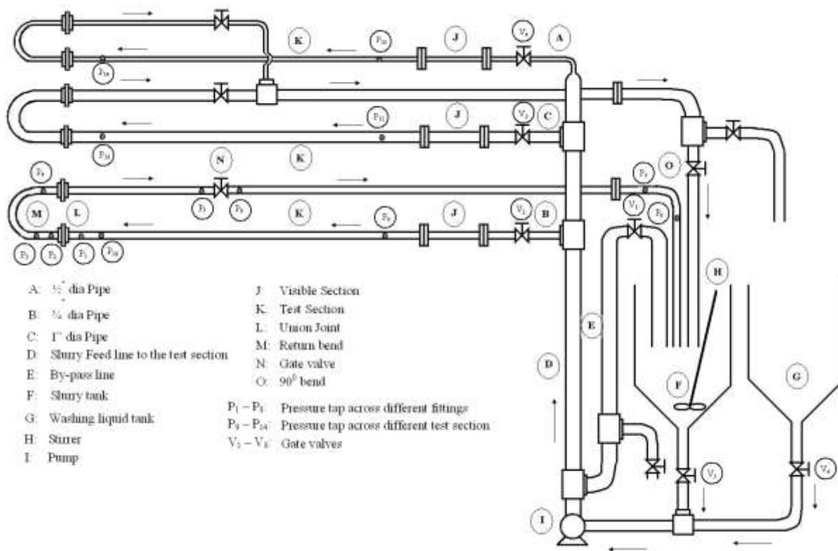
Figure 2 (b): Schematic diagram of experimental set-up for studding the rheological behavior of coal – oil-water – additive slurry
