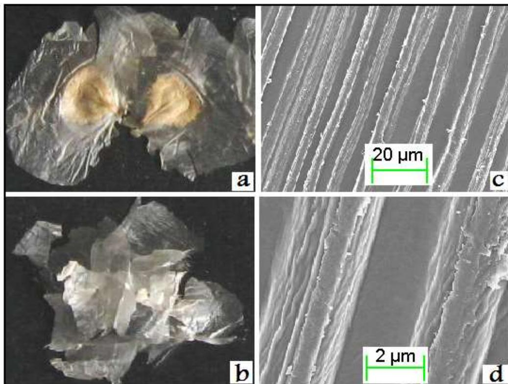
**Figure 1:** Photographs of ground dry cellulose films taken with digital camera (a) with seed and (b) without seed. (c) FESEM images of the film with (d) a magnified image of nanofibers
