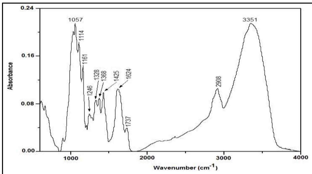
Figure 3: FTIR spectrum of dried isolated film
