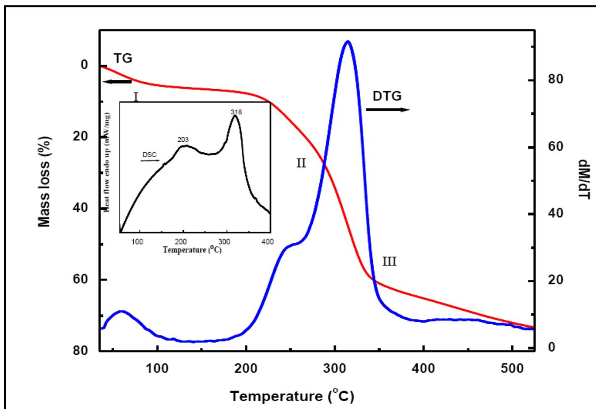
Figure 2: TG-DTG thermograms of film. DSC thermogram (inset) was obtained by measuring at 5 °C/min heating rate in N<sub>2</sub> atmosphere
