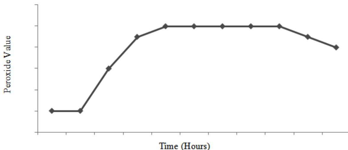
Figure 1: Peroxide formation and decomposition as a function of time
