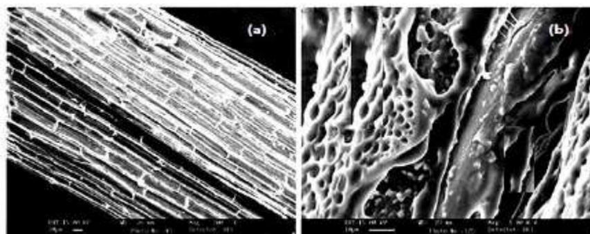
Figure 4: SEM of (a) Control jute fiber (b) Jute-TMS were carried out on Electron Microscopy Machine (LEO 435 VP)
