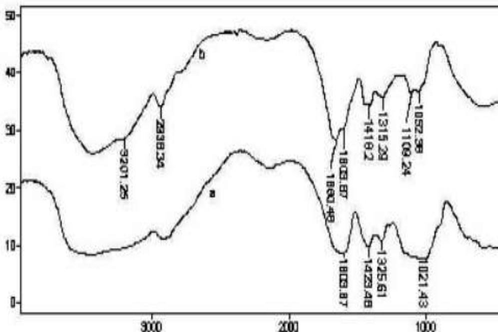
IR spectra of the control and grafted jute fiber were taken with KBr pellets on a Perkin Elmer Lamda-35 (USA) UV VIS spectrophotometer.
