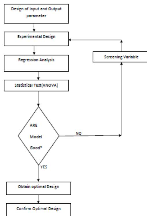
Figure 5: Flow chart for procedure of Response surface methodology
