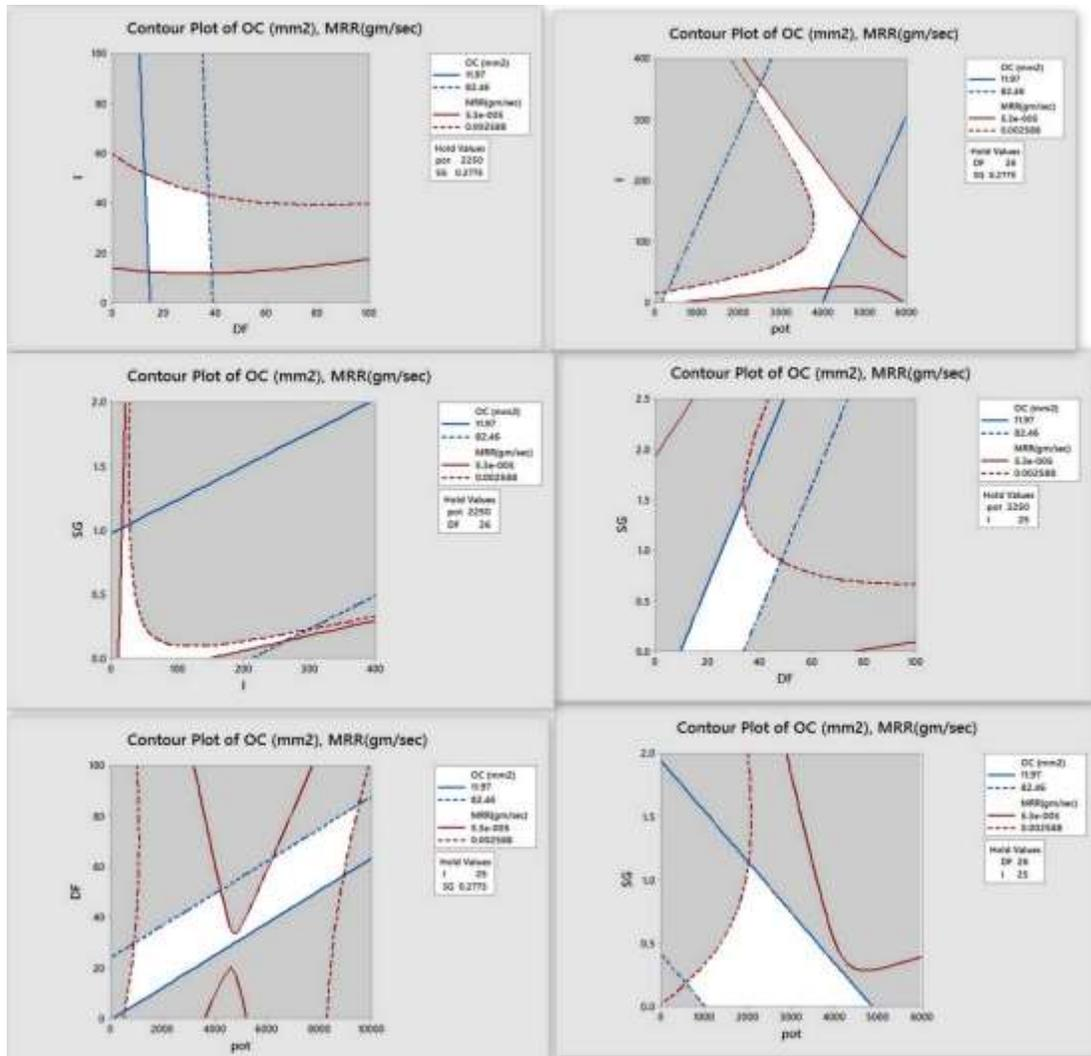
Figure 8: overlaid contour plots for MRR and Overcut (OC)
