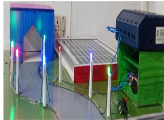
Figure 2: Hardware implementation of the prototype with the monitored panel and connected load.
