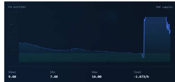
Figure 7: pH history over the same 360-sample window (mean 9.60, range 7.48–14.00, trend -1.673 /h). The step near the end of the window corresponds to the electrode being lifted from the sample during handling, and illustrates the range-plausibility flagging described in Section III.
