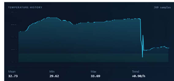
Figure 6: Temperature history over a 360-sample observation window, with mean, minimum, maximum and hourly rate-of-change statistics computed on the node (mean 32.73 °C, range 29.62–33.69 °C, trend +0.90 °C/h).
