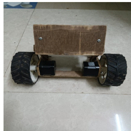
Figure 4: Robot prototype used for PID tuning
