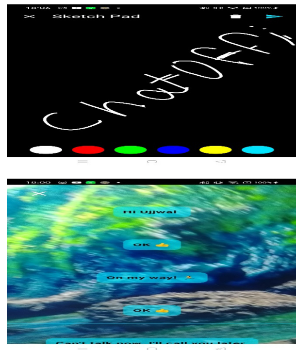
Figure 4: The integrated digital Sketch Pad allowing users to transmit hand-drawn graphical payloads over the mesh network.
