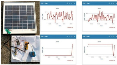
Figure 3: Field deployment of the monitored panel and the corresponding cloud dashboard.
