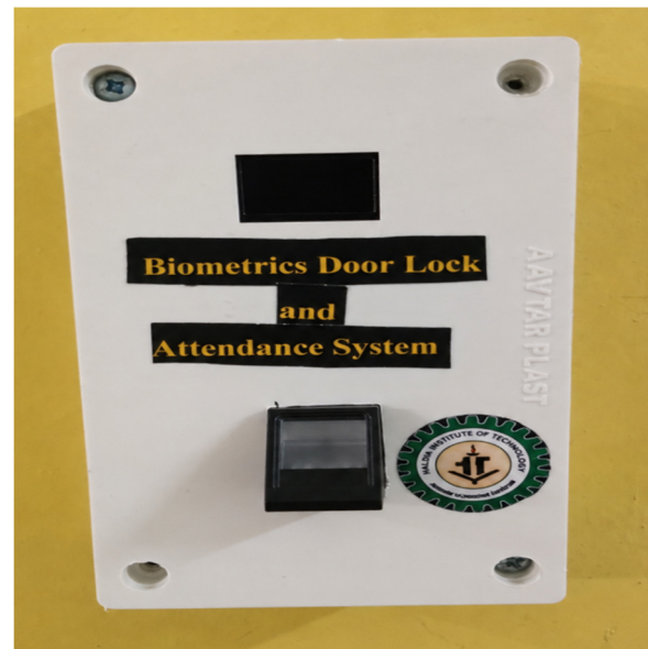
Figure 3: Biometric Access and Attendance control unit
