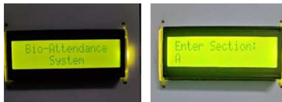
Fig. 4: LCD showing message for user
