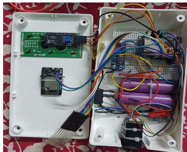
Fig. 1: Complete Circuit of Biometric Attendance System
